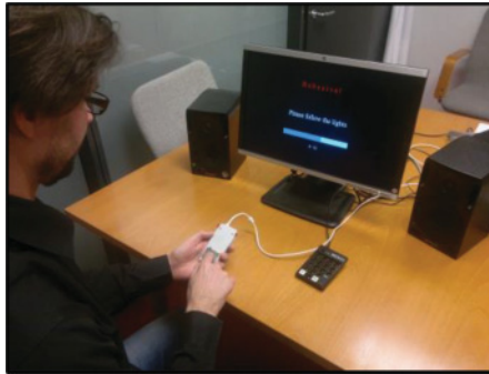
Fig. 5. Experiment setup. Participants held the Virtual Button Simulator in their nondominant hand and pressed the keys with their dominant hand. They responded with a modified keypad connected to a PC.
